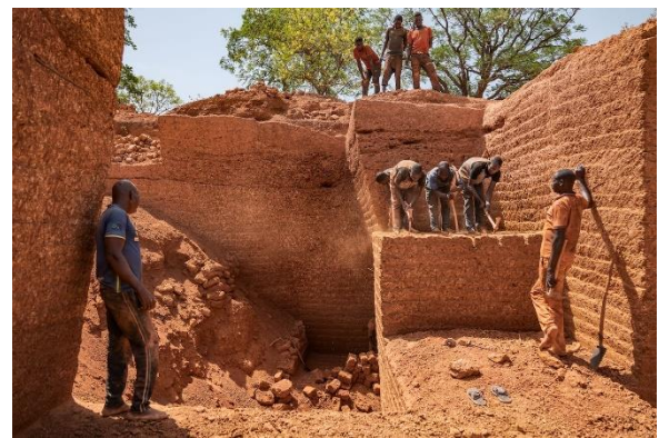
Workers at a quarry in Houndé, Burkina Faso, hammer laterite stone bricks from the solid ground. Mud bricks must be shaped before drying, but laterite can be extracted in rectangles. Both traditional building materials create much cooler structures than concrete, are cheaper, and require less energy to produce.
